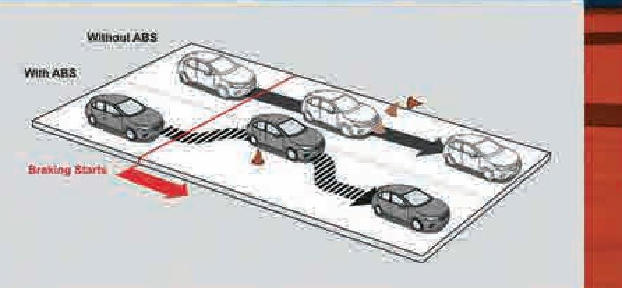
Anti Lock Brake System (ABS) with Electronic Brake-Force Distribution (EBD)
